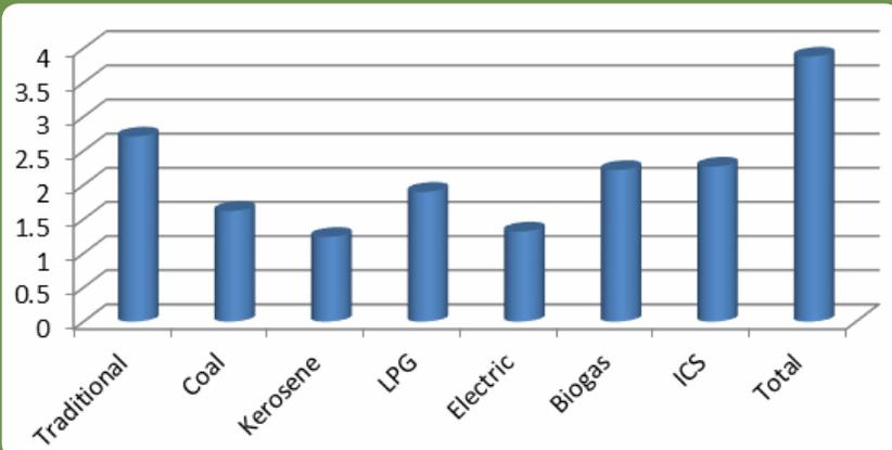
On average, households with traditional mud stoves used them for 2.71 hours per day (figure 2). Kerosene pump stoves were used 1.24 hours per day, LPG stoves for 1.9 hours per day and biogas stoves for 2.22 hours per day.
